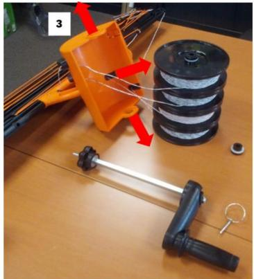
Now remove the reels out of the housing by gently stretching both sides of the housing a little apart (3).
