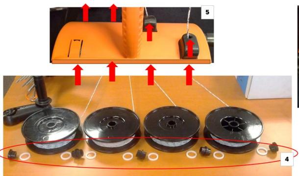
The reels now can be separated very easily from each other, remember the locations of the bearings and rings holding the reels together (4). Replace the reels with new ones by putting all the bearings and rings back in the same location as before.
